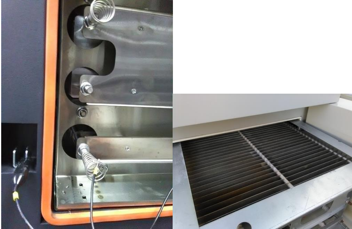
Fig. Discharge high voltage plates
