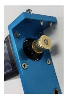
Place the belt "H' to the motor pulley. Then, fasten the frame back to the motor bracket with the 3 screws shown in Step 1.
