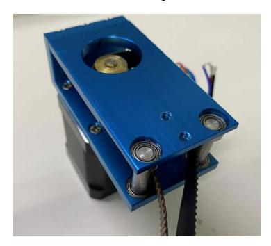
Fasten the motor bracket assembly with short screws to the bottom frame "A".
